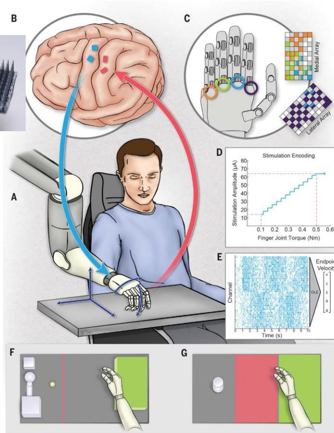
Figure 1 presents an overview of the bidirectional brain-computer interface (BCI) system. (A) The participant used an intracortical BCI to continuously control a robotic arm in five movement dimensions during each trial.
